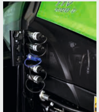
↑ Mid-mounted hydraulics ways for front implements.
