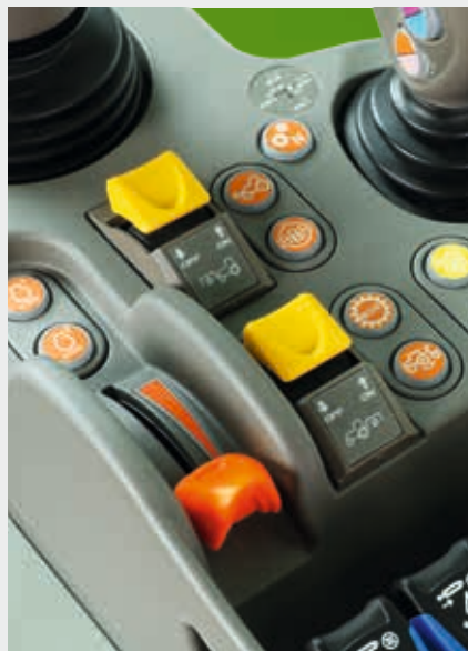
↑ Easy engagement of front and rear PTO through buttons on MaxCom armrest.
