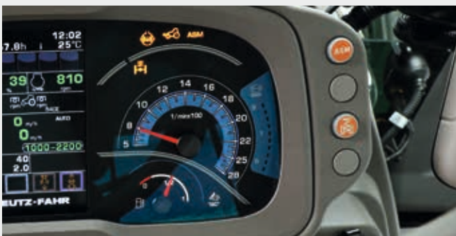
↑ ASM and front axle suspension activation.
