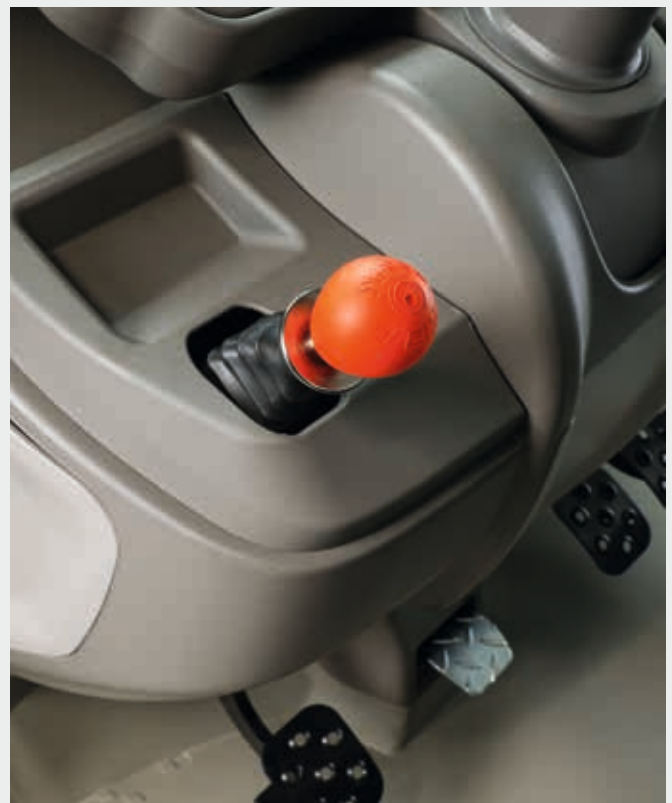
↑ Safe parking even in hilly conditions thanks to powerful HPB parking brake.
