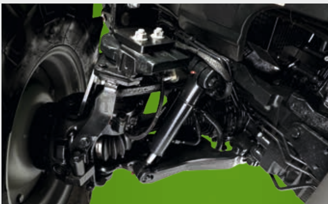
↑ Suspended front axle with front brakes.
