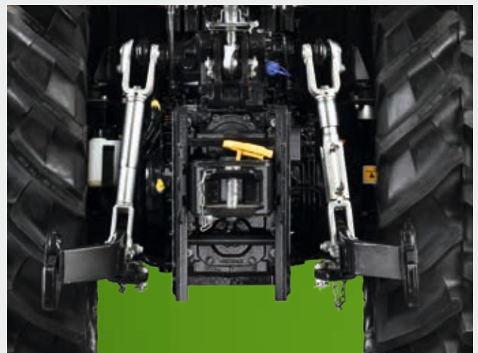
↑ Compact three-point hitch for narrow track.
