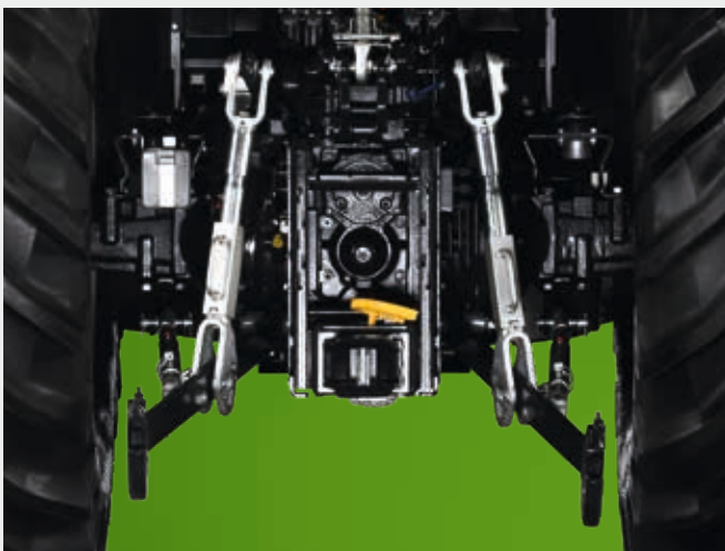
↑ Standard three-point hitch for higher lifting capacity.
