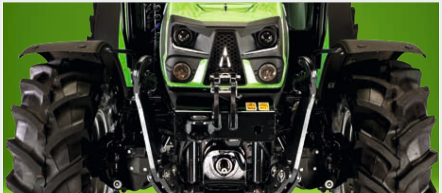
↑ 5D TTV models can be equipped with a front lift with 2,880 kg capacity and optional comfort package.
