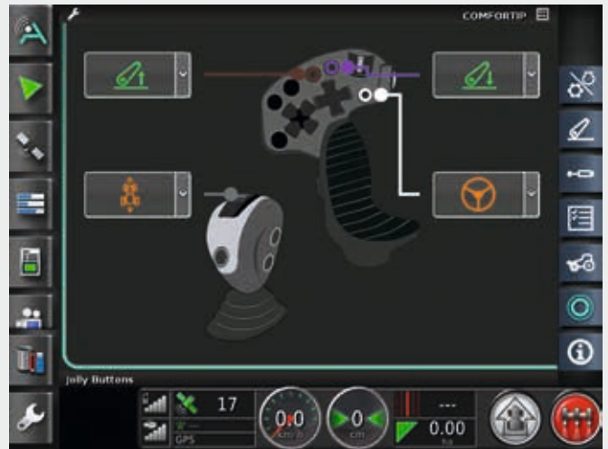
3 jolly buttons and 1 programmable thumbwheel.
