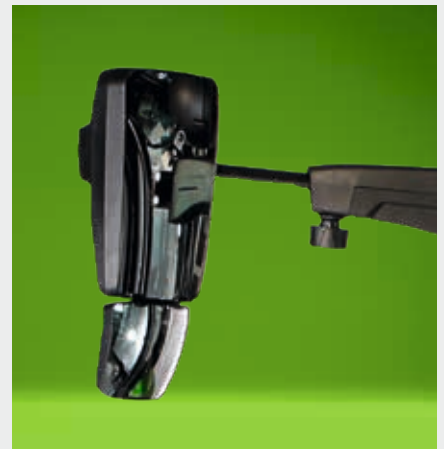
↑ Mirrors with electric adjustment and defrosting.
