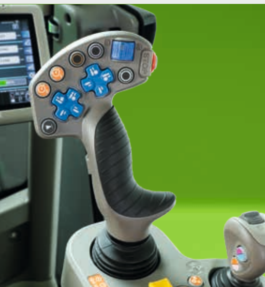
↑ MaxCom joystick for simple management of TTV transmission.
