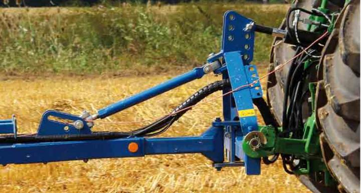
While working, the power traction kit gives additional weight from machine to rear
